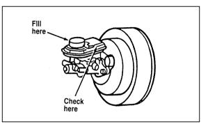
The anti-lock brake system fluid reservoir
